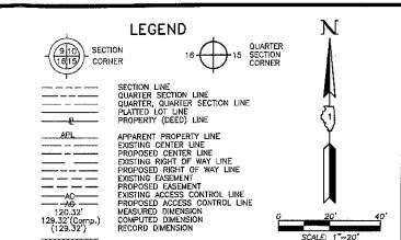
Bearings and Coordinates are referenced to the Illinois Coordinate System NAD 83(2011) East Zone.
